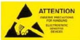
**WARNING:** White LEDs are made using a blue (GaN) die. GaN die is highly susceptible to Electro Static Discharge (ESD) damage, therefore proper storage, handling and manufacturing procedures need to be followed at all times. ESD damage can vary in its degree; from very subtle to catastrophic, and invariably will affect the LED's performance and life.
